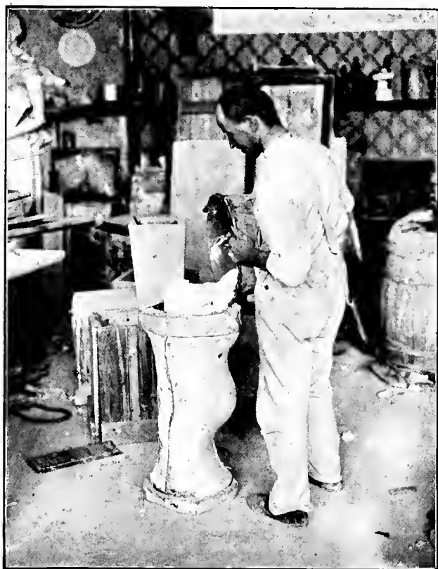
Fig. 67—Pouring the Glue into the Case and Around the Model
